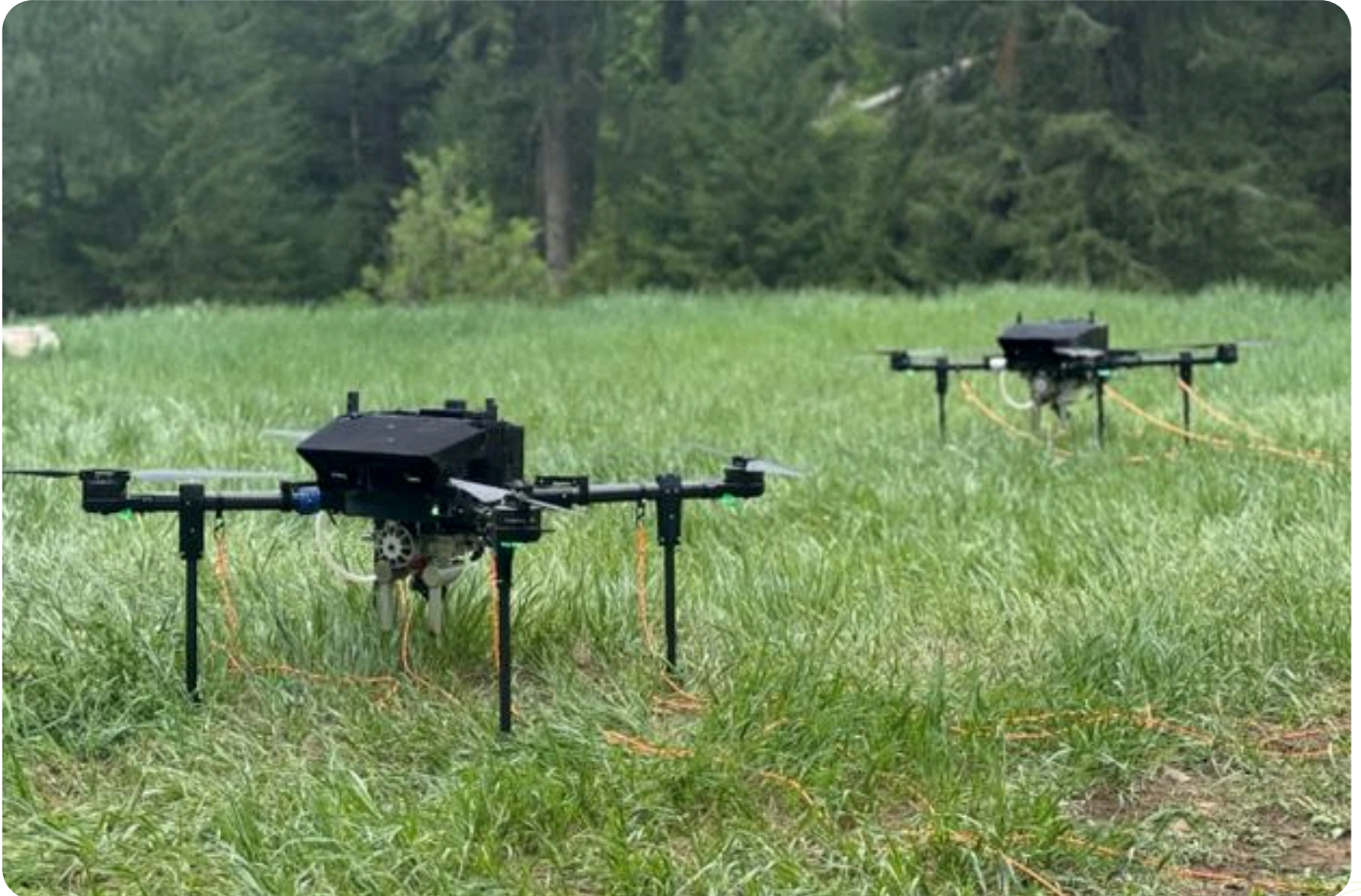
Figure 4: The Recon Lite hybrid. The multi-robot solution used in the Gull River survey.
